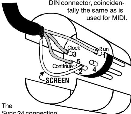
The Sync 24 connection cannot be made with a plain MIDI cable, as shown in the diagram above, it requires a pin-to-pin cable with pins 1, 2, 3 and 5 connected. Although they use the same type of connector, you should never connect MIDI sockets to Sync24 sockets.
