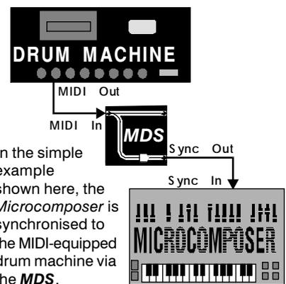
In the simple example shown here, the *Microcomposer* is synchronised to the MIDI-equipped drum machine via the *MDS*.
