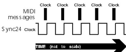
The *Philip Rees MDS MIDI to Sync24 Converter* listens to an incoming MIDI SRT clock stream and generates a corresponding Sync24 (DIN sync) format output. The *MDS* appears as a tempo slave to your MIDI system, and is a tempo master in Sync24. When you have installed your sync converter, your Sync24 device(s) should start, play in time, and stop automatically, by remote control from your MIDI master equipment.
